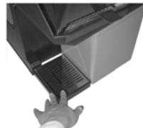
**Top/Fast Top:** Place the basket, remove the filter and the cover screen. Fit the feeding tube. Replace the cover screen and the filter. Finally place the peel buckets and the juice tray.
