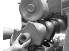
Remove the squeezer drum by unscrewing the
